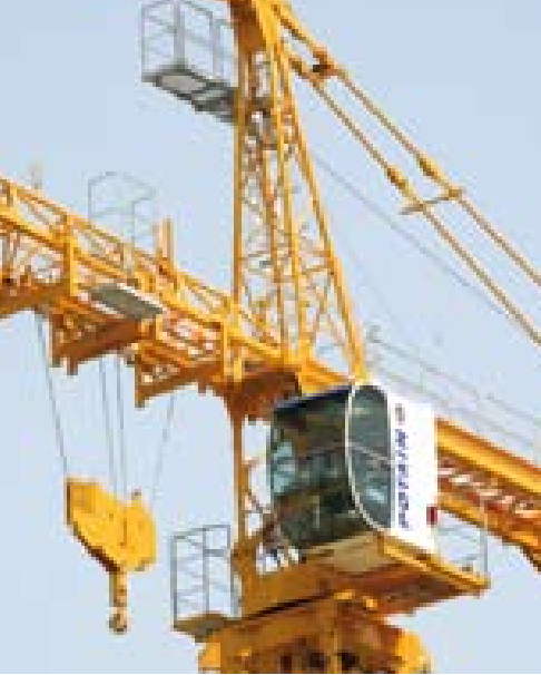
The cabin is on the same side as the trolley basket.
