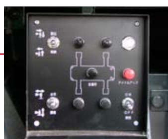
Outrigger controls on carrier and upper works.
