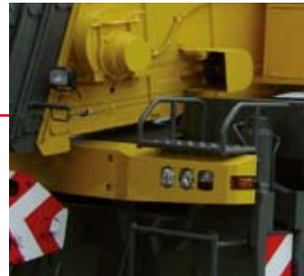
Cab roof and lower turntable lights.
