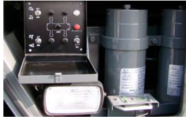
Outrigger spot lights for each outrigger.
