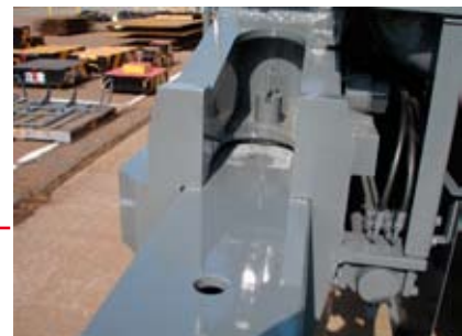
Outrigger lock pins Outrigger extension potentiometer.
