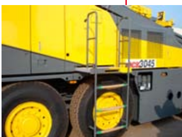
Platform and access ladder for fueling.
